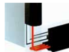
Detail heating element on floor
